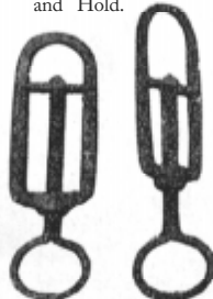
Fig. VI. Screw-Keys Which Held the Man-Trap Springs While the Trap Was Being Set.
